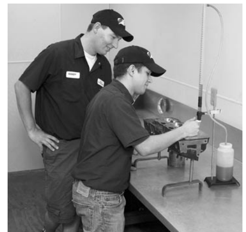
Checking chamber volume
