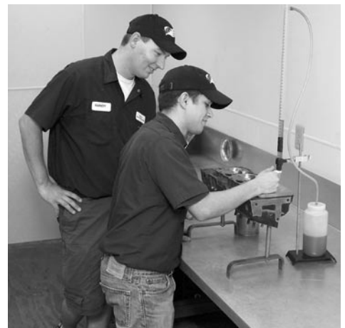
Checking chamber volume
